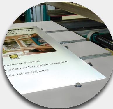
Aluminum vacuum table shown with pneumatic gripper cut-outs and optional disappearing registration guides features easy loading with superior substrate holddown.
