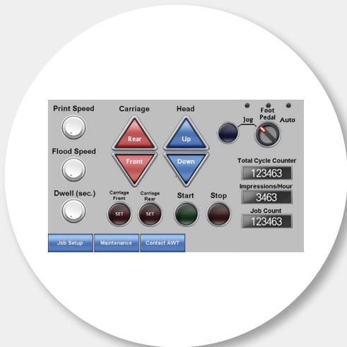
The touchscreen allows the operator to control a variety of functions such as print and flood speeds, carriage and print head position and cycle counts, with a simple touch.
