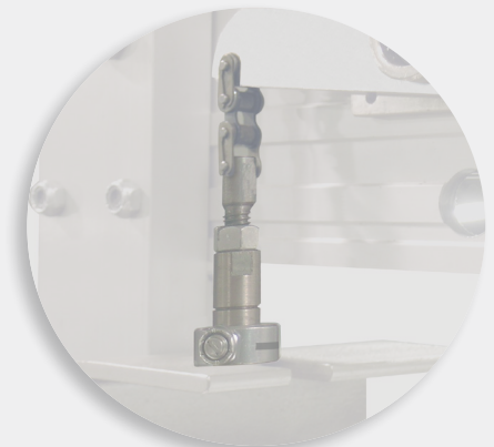
Four-point off-contact control enables "0" off-contact for printing with high-tension screens.
